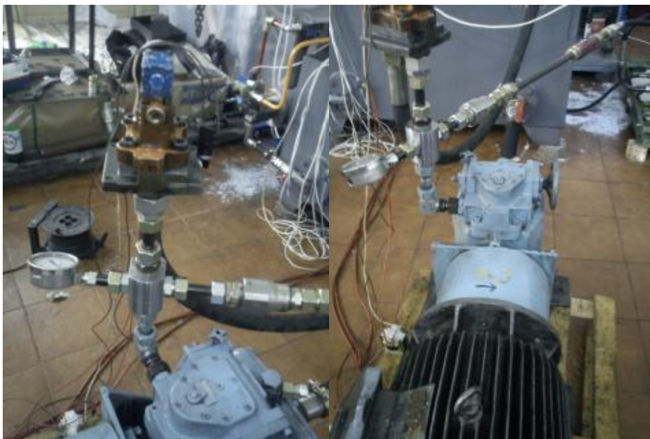
Standuri testare pompe hdraulicice
